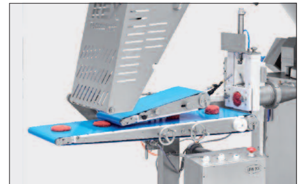
Cevapcici shaping by flow divider & form cutter
