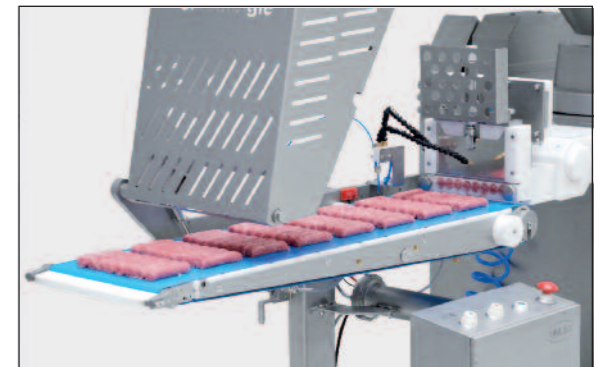
Cevapcici shaping by flow divider & form cutter
